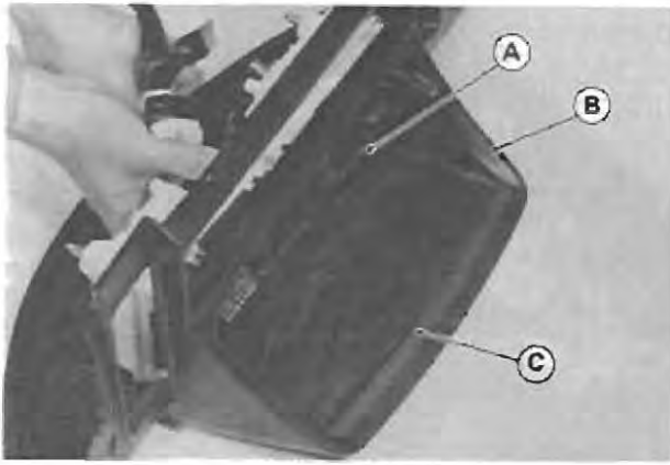
A. Meter and Gauge Assembly C. Seal Trimming B. Meter Assembly Cover
