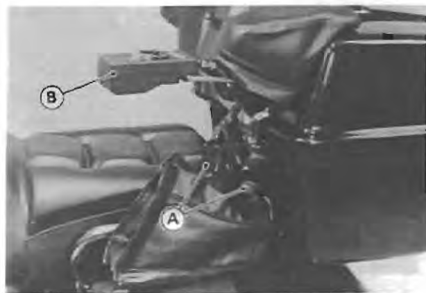
A. Connectors B. Passenger Switches
