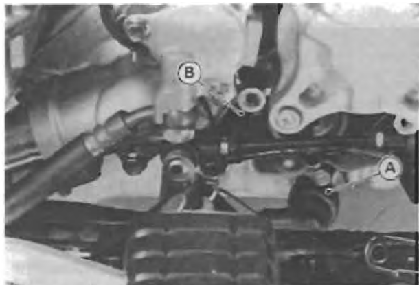
A. Oil Pressure Switch B. Neutral and Overdrive Switch
