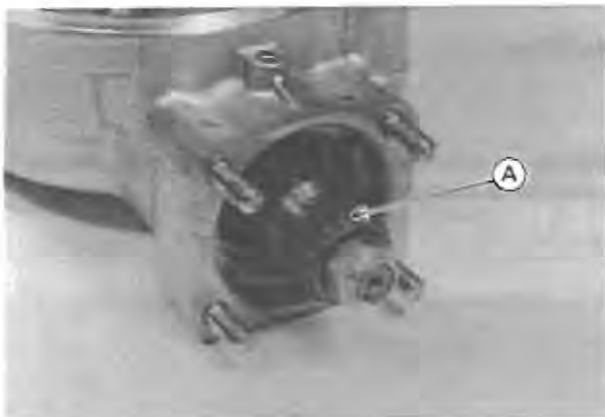
A. Check splined portion.
