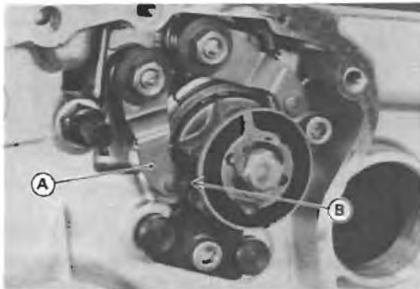
A. Neutral Positioning Lever B. Neutral Detent
