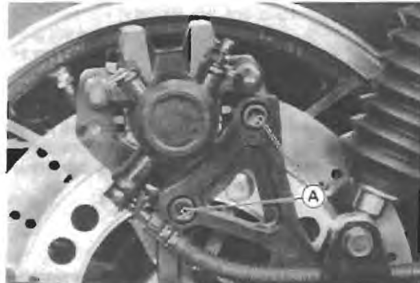
A. Caliper Mounting Bolts
