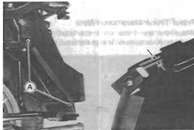
A. Rear Fender Rear Mounting Bolts
