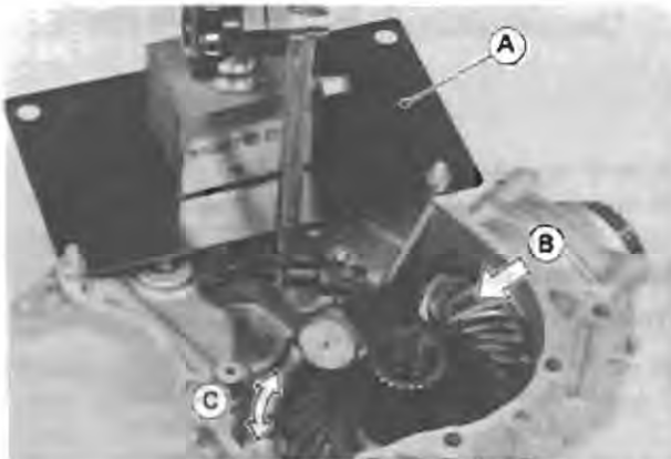
A. Holder: 57001-1049 B. Hold the driven gear.
