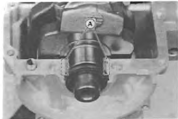
A. Do not apply a liquid gasket here.
