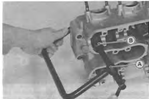
A. Valve Spring Compressor Assembly: 57001-241 B. Adapter: 57001-1019
