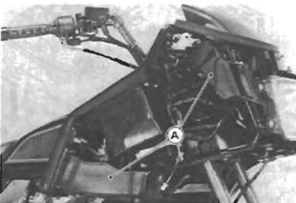
A. Air Ducts
