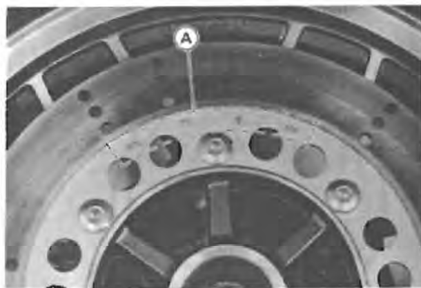
A. Minimum Thickness Marking
