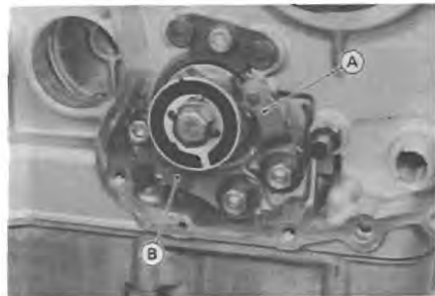
A. Neutral Positioning Lever B. Gear Positioning Lever
