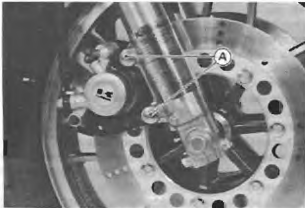
A. Caliper Mounting Bolts
