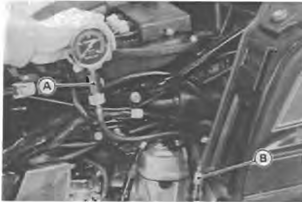
A. Compression Gauge: 57001-221 B. Adapter: 57001-1183
