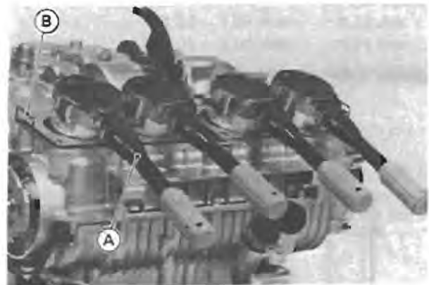
A. Piston Ring Compressor Assembly: 57001-1094 B. Piston Base: 57001-149
