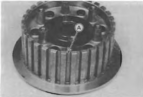
A. Clutch Hub Spline
