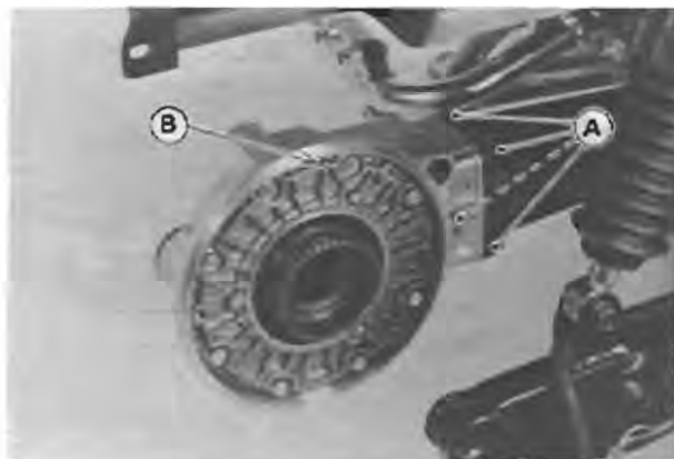
A. Final Gear Case Mounting Nuts B. Breather Hole
