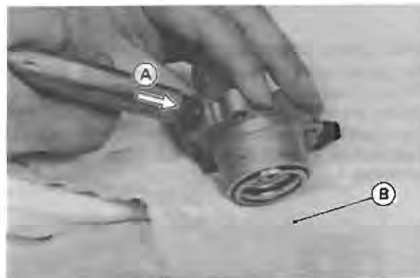
A. Apply compressed air. B. Cloth
