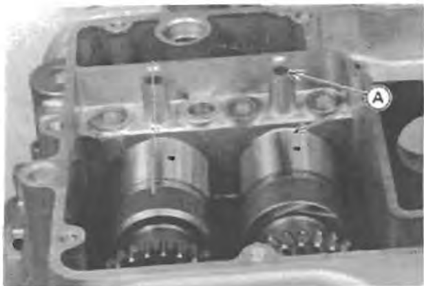
A. Align mark with hole center.
