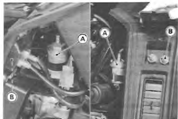
A. Oil Separator B. Air Valve
