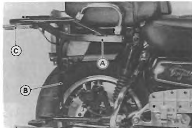
A. Travel Trunk Bracket C. Antenna Bracket B. Saddlebag Bracket
