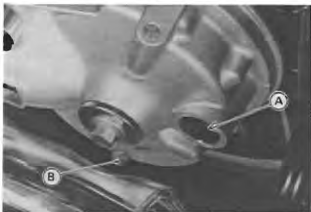
A. Filler Opening B. Drain Plug
