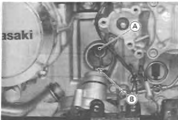
A. Oil Pump Shaft Projection B. Water Pump Shaft Slot
