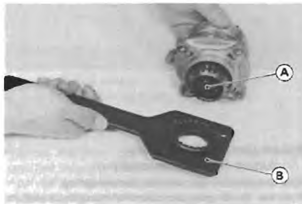
A. Driven Gear Bolt B. Driven Gear Holder: 57001-1027
