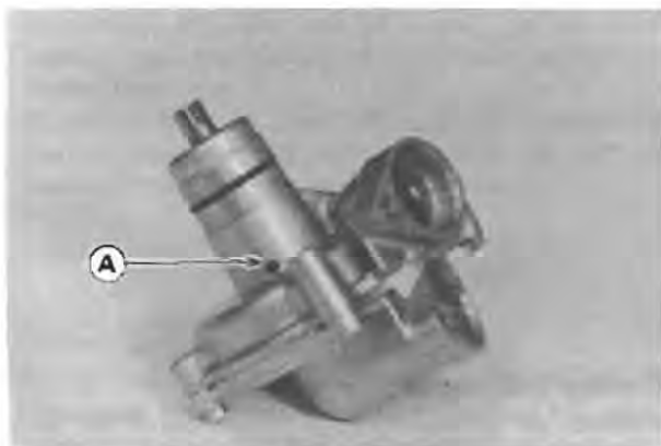
A. Drainage Outlet Passage at the bottom of the pump body
